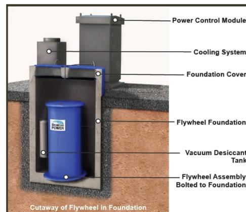
Figure 7 - Typical SmartBox PCM and Flywheel installation
