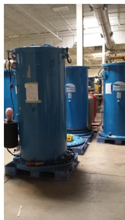
Figure 4 - FES rotor package
