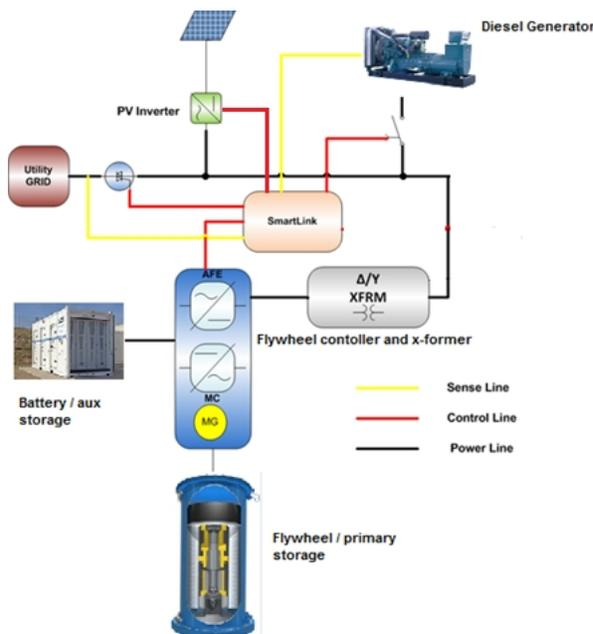
**Figure 5 - SmartBox MicroGrid typical configuration**
